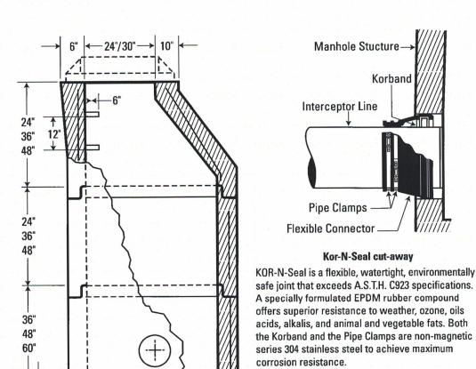
DESIGN SPECIFICATIONS CONFORM TO: "PRECAST REINFORCED CONCRETE MANHOLE SECTIONS – A.S.T.M. DESIGNATION C478, LATEST REVISION."
